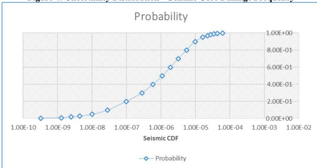
**Figure 5: Uncertainty Distribution – Seismic Large Early Release Frequency**
