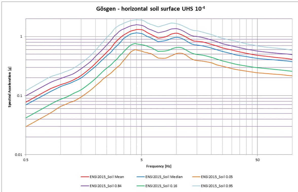
**Figure 2: Seismic Hazard Curve (PGA-100Hz) – ENSI 2015**
