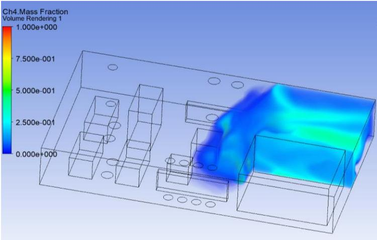
**Figure 5 CH4 velocity field from a dispersion simulation after a release in the central area**
