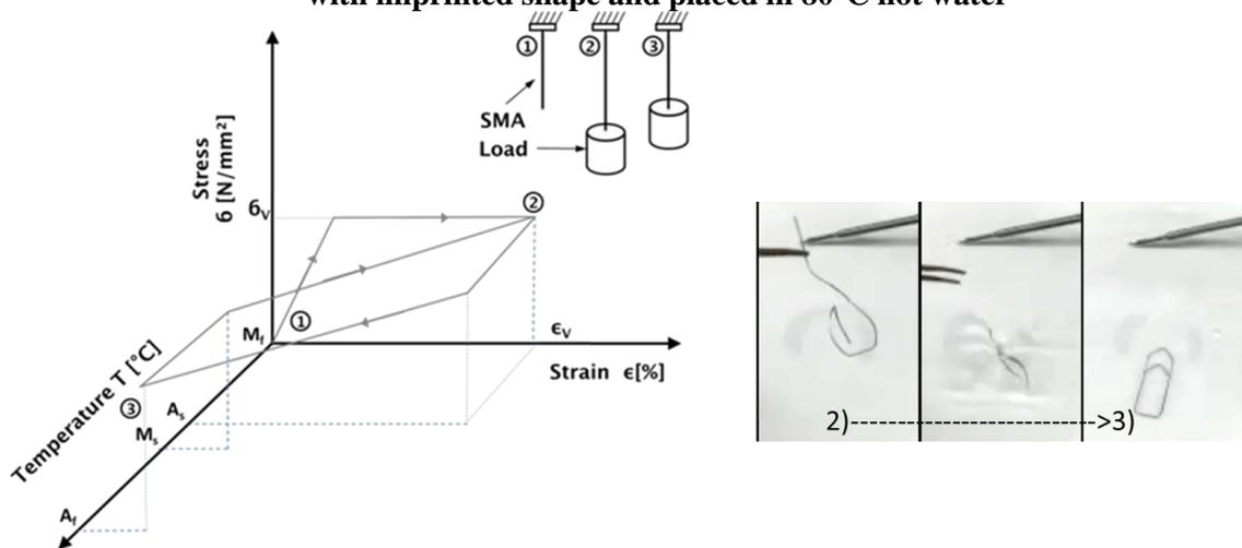
Today's SMA actuators can be found e.g. in small valves in automobiles [2], auto-focus systems in mobilephone-cameras [3] and thermal regulators for building automation [4]. Earlier publications [5] presented valve drives like the quench-valve. In this application the SMA wire quenches a flexible tube affecting the flow control of the fluid.
