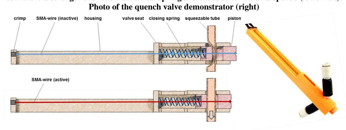
While there are striking advantages of SMA actuators concerning miniaturization and simplification, the development-time of SMA actuators is one of the major obstacles in this field. Due to the thermal characteristic, the resetting time of an SMA actuator corresponds the cooling time from the  $A_f$  to  $M_f$
