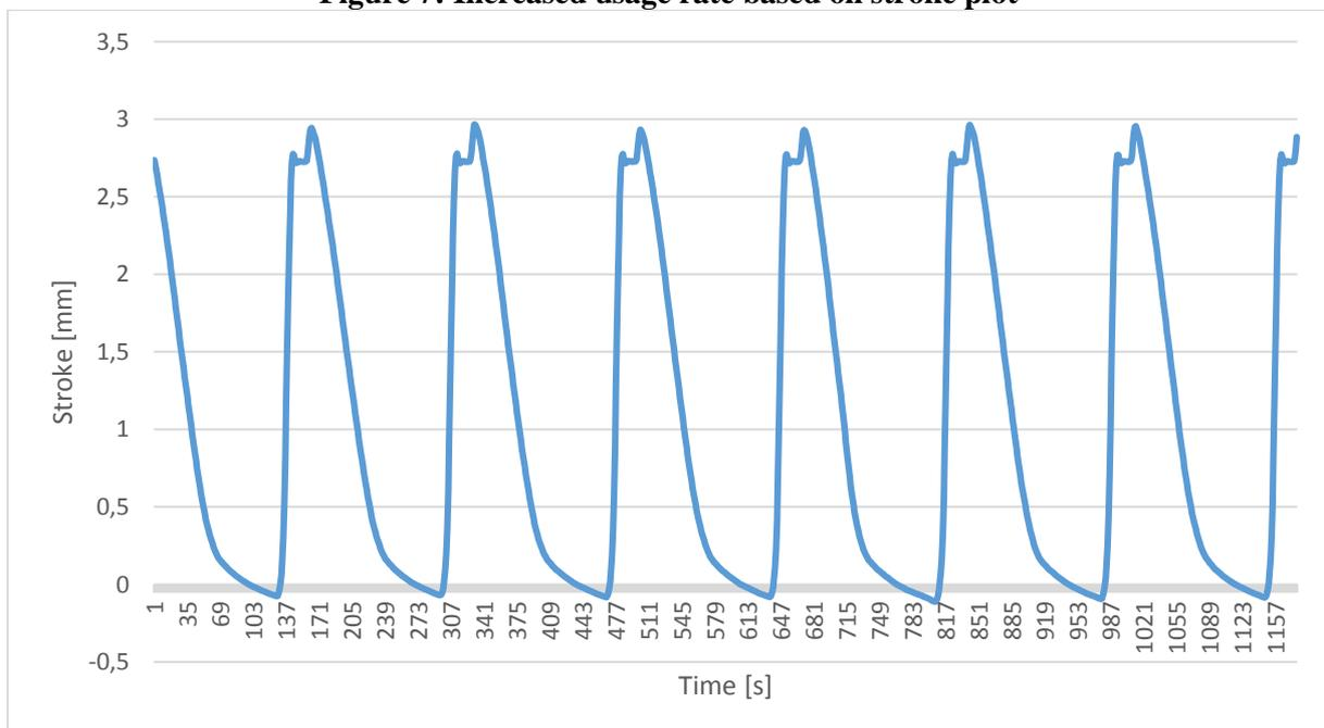
Obviously, the presented example shows only several cycles within 1200 seconds out of an entire test which is considered for 300.000 cycles. Nonetheless, the entire test is recorded in the exactly same manner.
