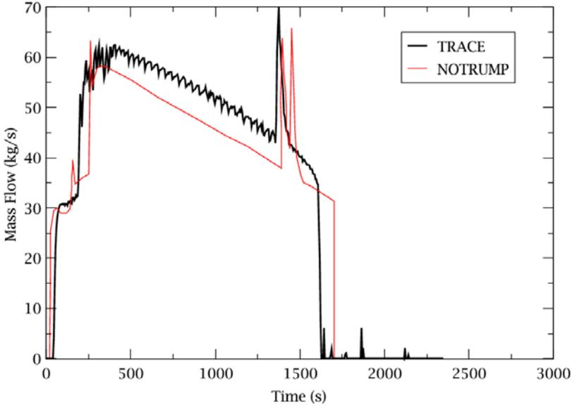
**Figure 7: DVILB low magin sequence. IRWST injection flow rate. TRACE vs NOTRUMP**
