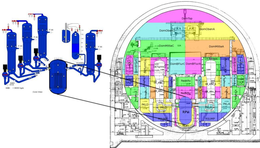
In addition, the ventilation channels below the surface of the reactor cavity bottom are considered as well. Thus, two modes of cavity rupture are possible to transfer molten material into the next cavity (“gap volume”). Between the latter one and the sump cavity there are dampers within the support shield whose lower edges are located very low above the bottom of this cavity. So there is only a certain small amount of corium necessary to trigger this rupture mode of the second cavity.
