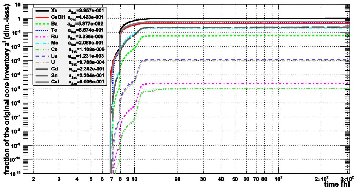
According to the explanation above the significant release into the environment starts with the large-scale deflagration in the annulus. The values at the end of the calculation are given in Table 4. For example, the fraction of the most volatile MELCOR group from the original core inventory is
