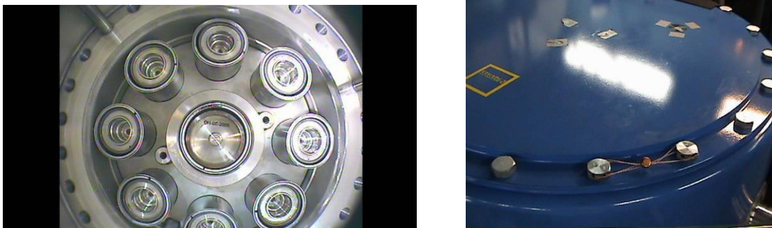
Figure 5. Pictures of CASTOR® KNK, basket with 9 cans and lid with seal
