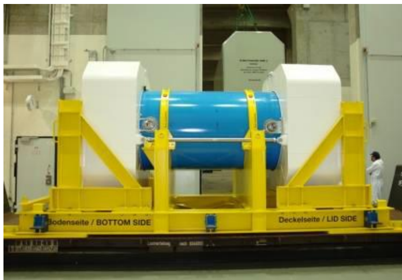
Figure 7. Cask on the transport frame
