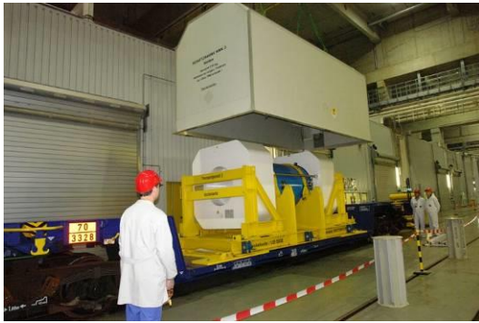
Figure 8. Cask handling at ZLN with horizontal and vertical lifting beam
