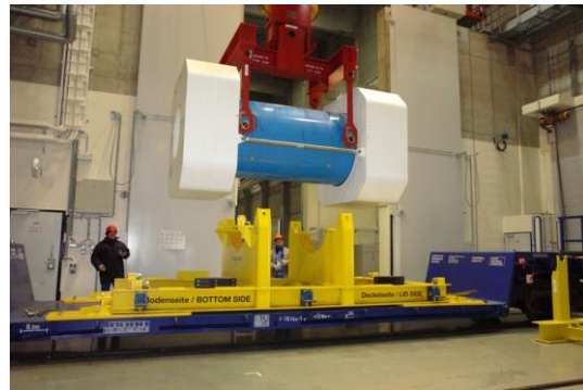
Figure 8. Cask handling at ZLN with horizontal and vertical lifting beam
