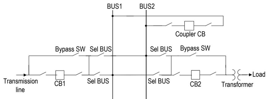
**Figure 4:** Double Bus and Five Switches
