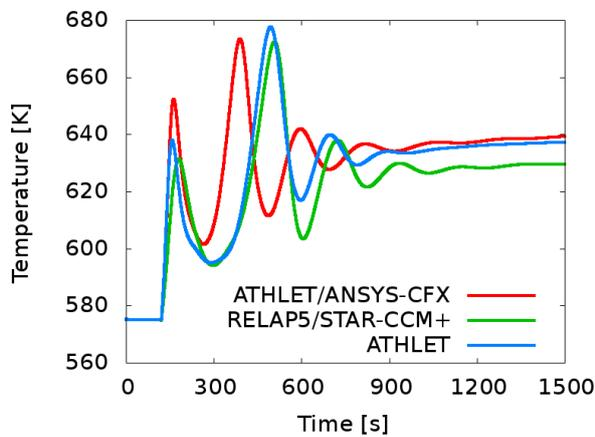
**Fig. 8: Temperature at the test section outlet**
