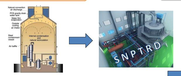
Passive Containment Cooling System: (height scale 1/8) **CERT(Containment safety vErification via integRal Test)**
