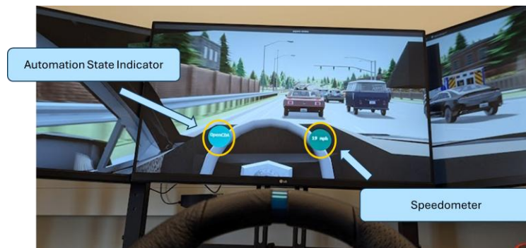
169 170 Figure 2: Experimental Setup - View from the driver's seat 171
