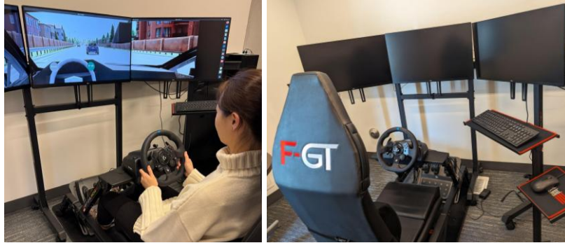
Figure 1: The driving simulator setup and the virtual driving environment OpenCDA
