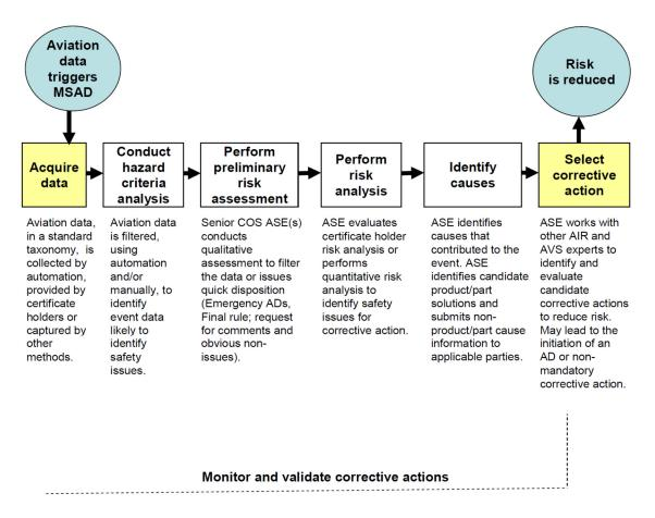
**FIGURE 2.1** The Monitor Safety/Analyze Data (MSAD) process. SOURCE: FAA Order 8110.107A. NOTE-- AD: airworthiness directive, AIR: Aircraft Certification Service, ASE: Aviation Safety Engineers, AVS: Aviation Safety, COS: continued operational safety, MSAD: Monitor Safety/Analyze Data.
