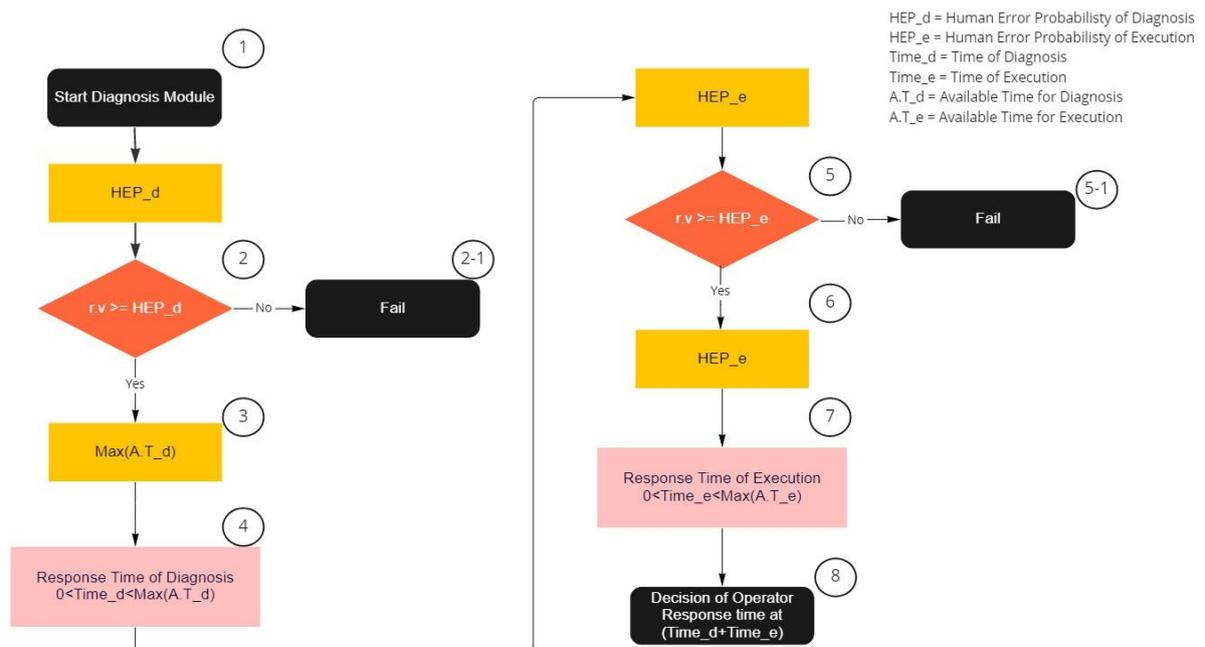
Fig 4. Algorithm for Operator Response Time Model
