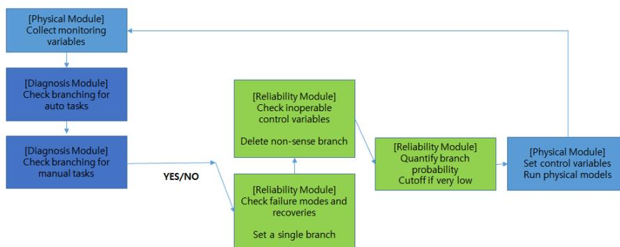
**Fig 3. Algorithm for Single-Branch Mode**
