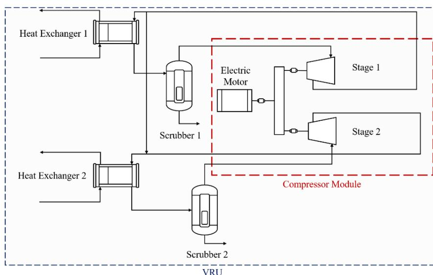
**Figure 2: Simplified Diagram of Vapor Recovery Unit.**
