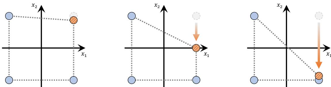
**Figure 5: Graphic representation of the  $2^2$  test plan when the fourth parameter combination is omitted (left), repeated (center); or when all parameter combinations are superimposed with a normally distributed scattering around their orthogonal position (right).**
