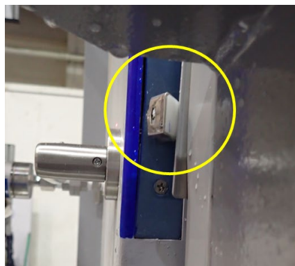
Fig.6. Damage of Latch bolt and flash bolt after tests
