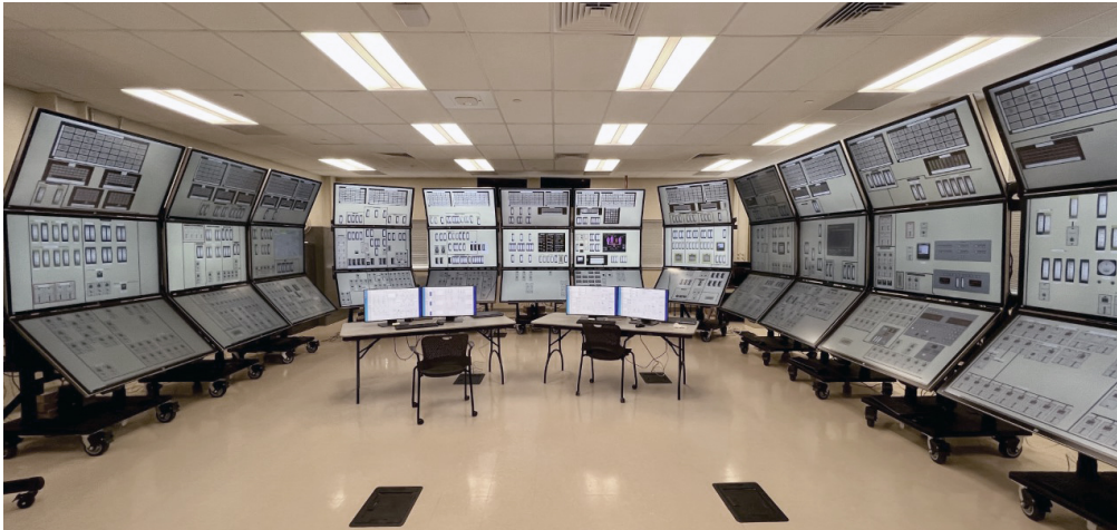
Figure 1: HSSL with the GSE GPWR Control Boards Displayed Virtually on Adjustable Bays
