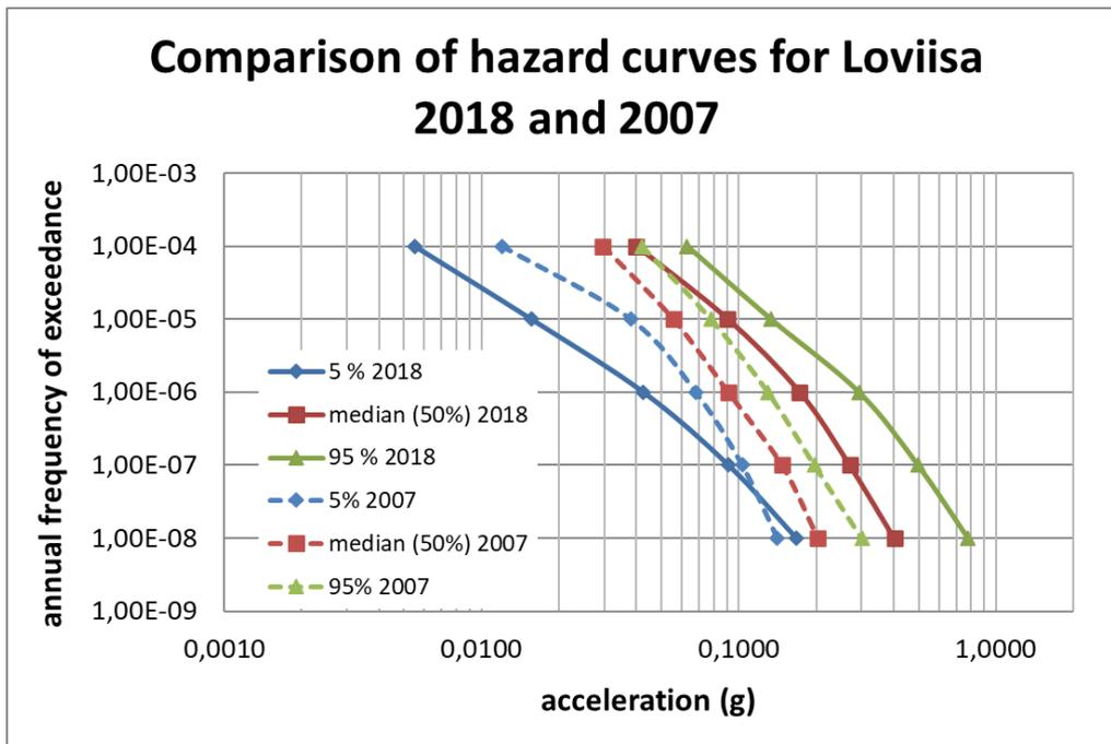
**Figure 2: Comparing 100 Hz hazard curves for Loviisa NPP site. Comparing results from probabilistic seismic hazard assessments 2018 and 2007 [4].**
