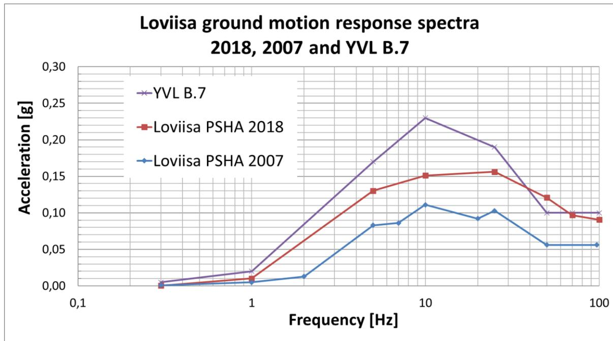
**Figure 1: Loviisa NPP 2018 site specific ground motion response spectra compared to probabilistic seismic hazard assessment (PSHA) conducted at 2007 [4] and YVL B.7 design spectrum [8] scaled to PGA 0.1 g with annual frequency of exceedance of 1E-5/a.**
