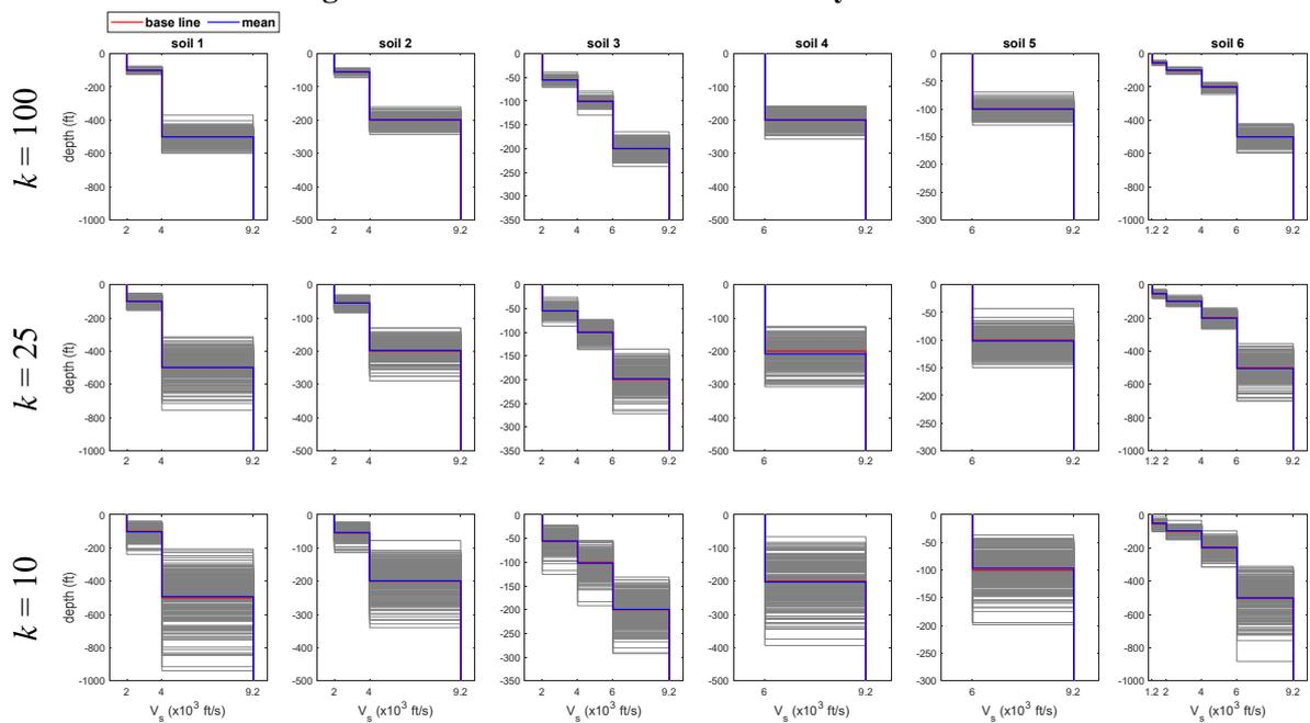
**Figure 4: Soil-amplification functions with the variability of the layer thickness**
