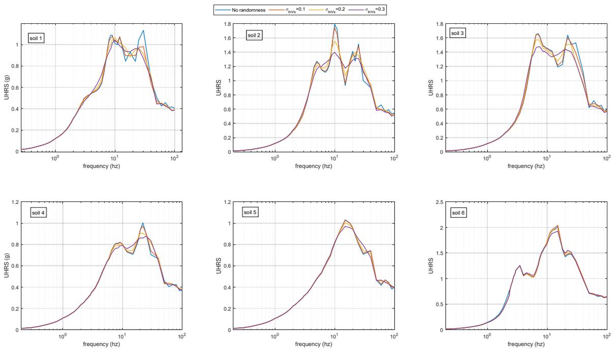
**Figure 10: Ground motion response spectra with the variability of the low-strain shear-wave velocity**
