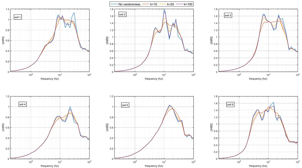
**Figure 6: Ground motion response spectra with the variability of the layer thickness**
