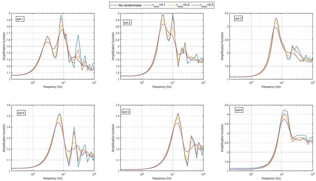
**Figure 9: Uniform hazard response spectra with the variability of the low-strain shear-wave velocity**
