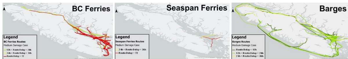
Figure 8: Illustrative output of the maritime route disruption model for a plausible M9.0 Cascadia subduction zone earthquake, applied to maritime shipping routes derived from AIS data; based on [9]
