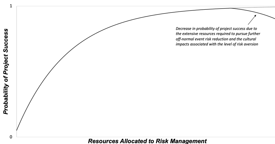
Figure 2: Probability of Project Success versus Resources Allocated to Risk Management when Accounting for Detrimental Effects
