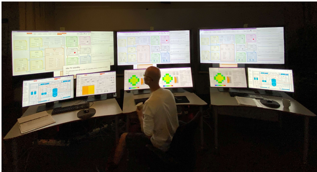
Figure 4: The basic principle iPWR simulator setup in the Halden Future Lab
