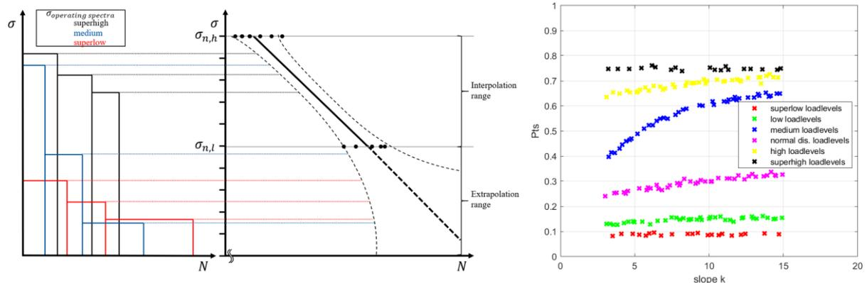
Figure 8 on the right shows that at low test levels, the correspondingly lower operating load spectra achieve a higher  $P_{tS}$  than the high operating load spectra. The influence of the slope  $k$  on the  $P_{tS}$  is lower. For the medium operating load spectrum, the slope  $k$  now even slightly reduces the achievable  $P_{tS}$ . Figure 8 on the left therefore shows that  $P_{tS}$  decreases the further away the operating load spectrum is from the test loads.
