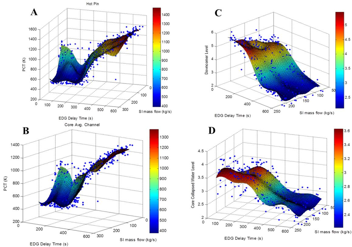
Fig. 4. Simulation data and GPM response surfaces for A) hot pin PCT, B) core average channel PCT, C) minimum downcomer collapsed water level, and D) minimum core collapsed water level.
