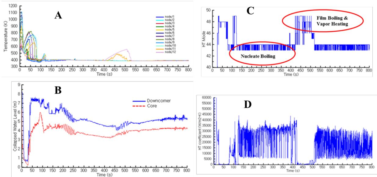
Fig. 2. Plant parameters during injection phase of LBLOCA. A) Axial clad temperature profile of hot pin. B) Collapsed water level in downcomer and core. C) MARS model active heat transfer mode and boiling regime. D) Heat transfer coefficient calculated by MARS code from the outer clad surface of a hot pin to the coolant.
