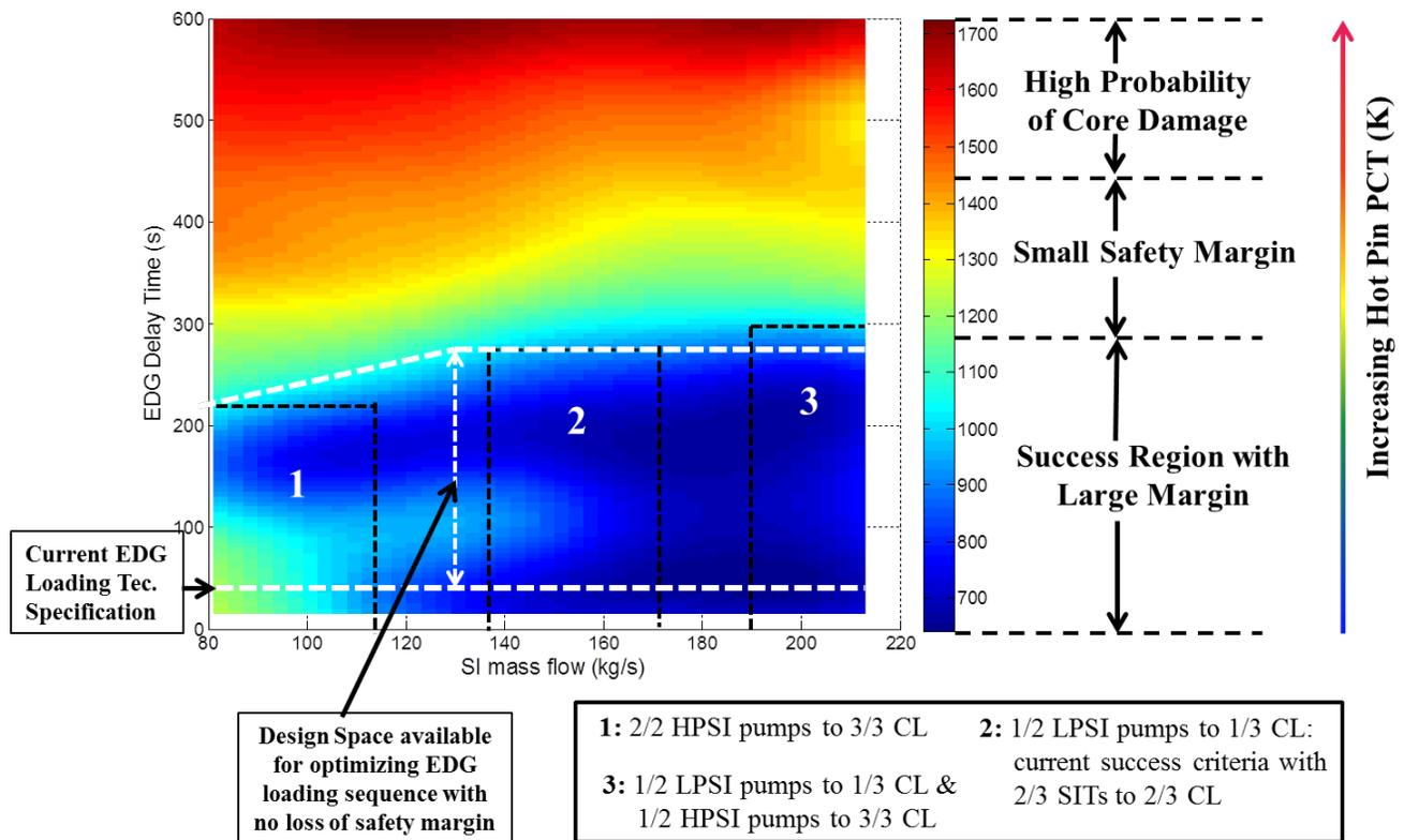
Fig. 6. Success criteria map for LPSI+HPSI pump configurations and EDG loading sequence timing with quantification of the safety margin.
