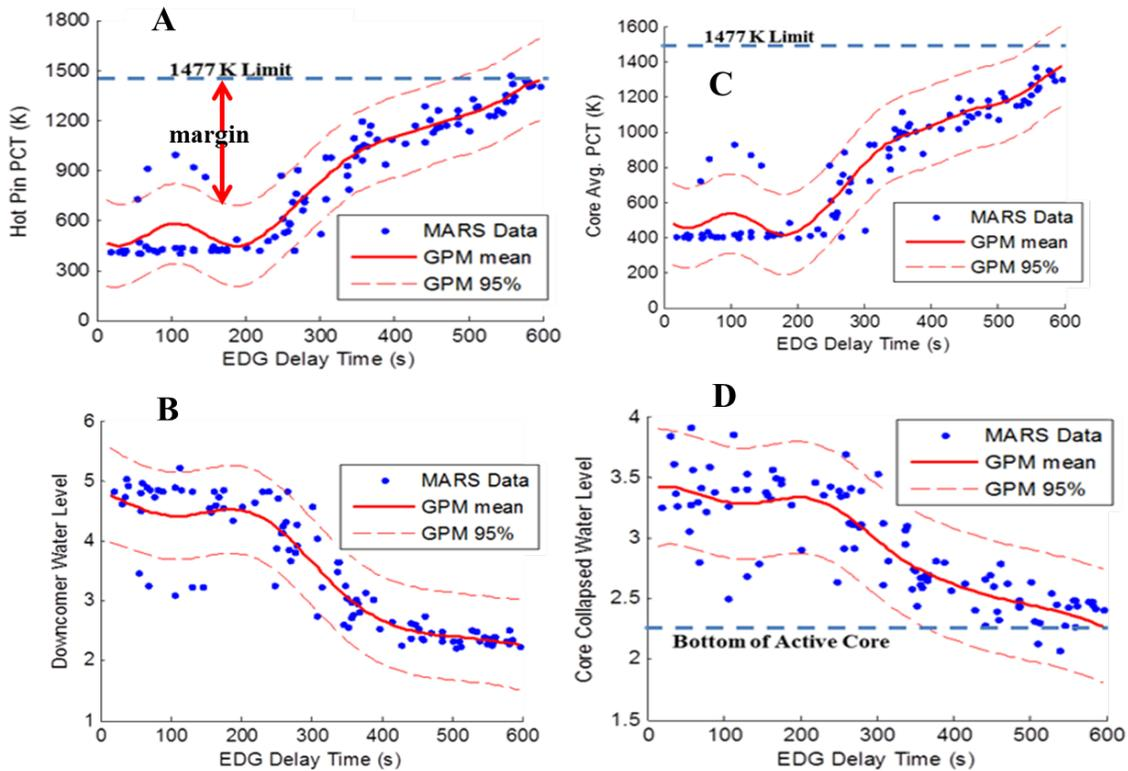
Fig. 5. Uncertainty bounds for A) Hot pin PCT. B) Core average channel PCT. C) Minimum downcomer collapsed water level. D) Minimum core collapsed water level.
