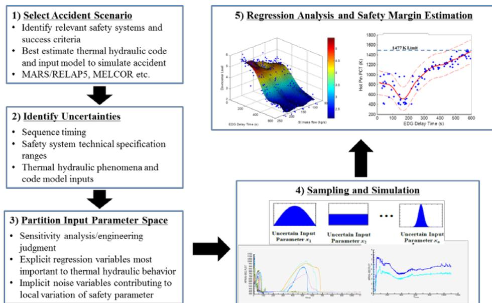
Fig.3. Flowchart of Gaussian process model regression methodology for safety margin estimation.
