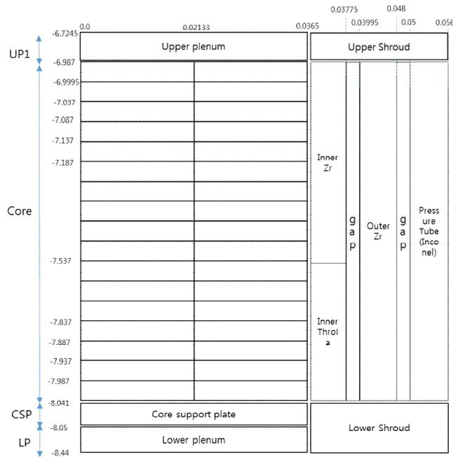
Fig.4 Node system of COMPASS
