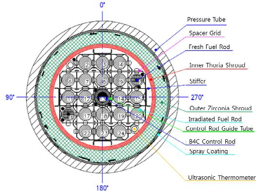
Fig. 2 Cross-sectional view of test bundle [9]
