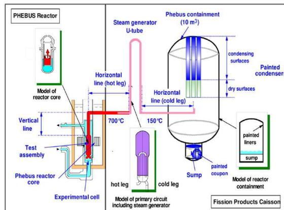
Fig.1 Schematic diagram of PHEBUS FPT3 [9]
