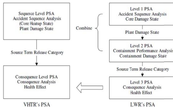
Fig. 1. Modified PSA process for VHTR (Ref. 4)
