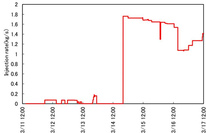
Fig. 2. Water injection rate from fire engine in water injected case
