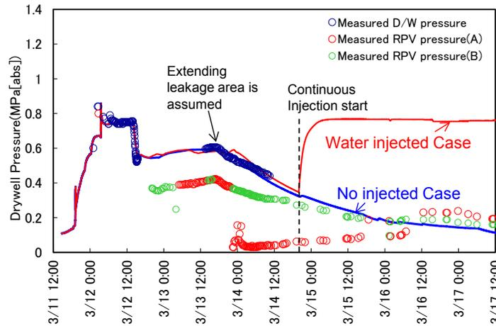
Fig. 3. Calculated PCV pressure
