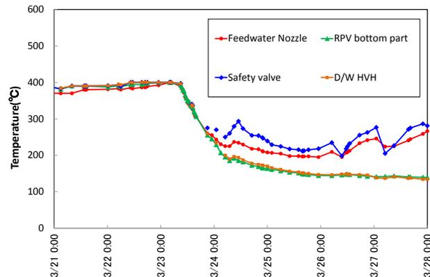
**Fig. 1. Measured internal PCV pressure and temperature in Fukushima Dai-ichi Unit 1**
