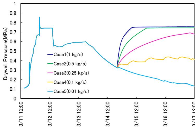
Fig. 5 Drywell pressure in sensitive analysis
