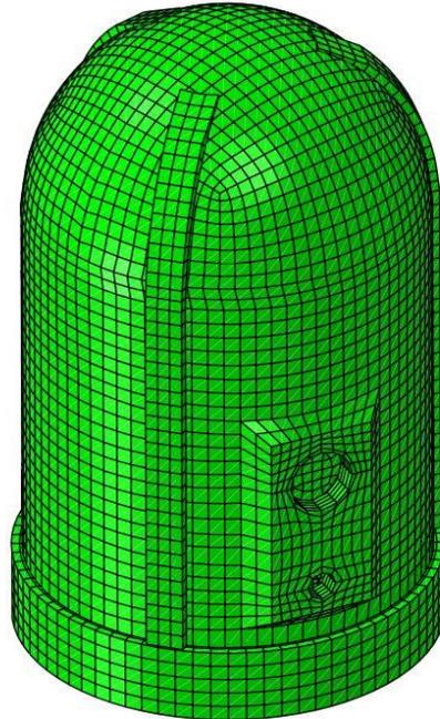
Fig. 1. The finite element model of the prestressed containment building.
