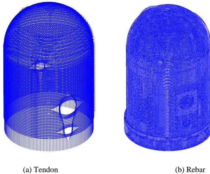
Fig. 2. The shape of finite element model of rebar and tendon
