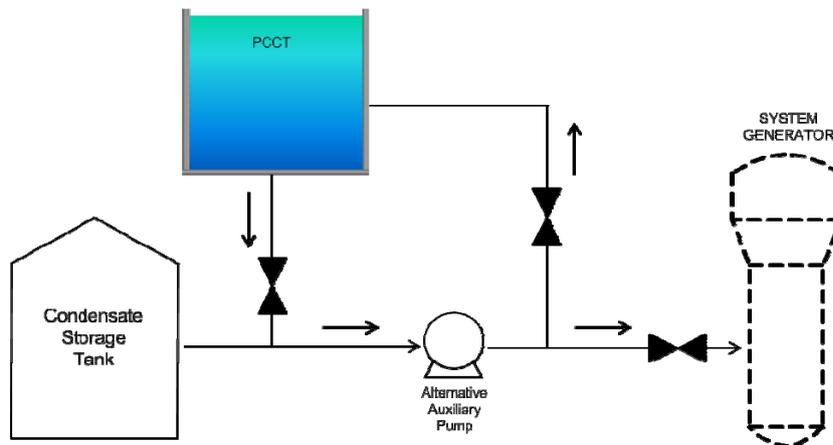
Fig. 3. Outline of Alternative Auxiliary Pump
