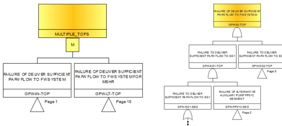
Fig. 4. Examples of Top gate of PAFS in Fault Tree
