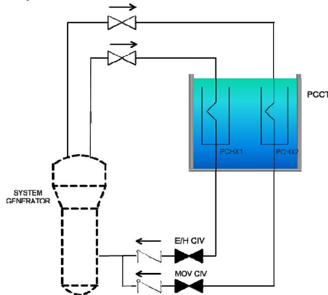
Fig. 1. Outline of Condensate Cooling Water Supply Loop
