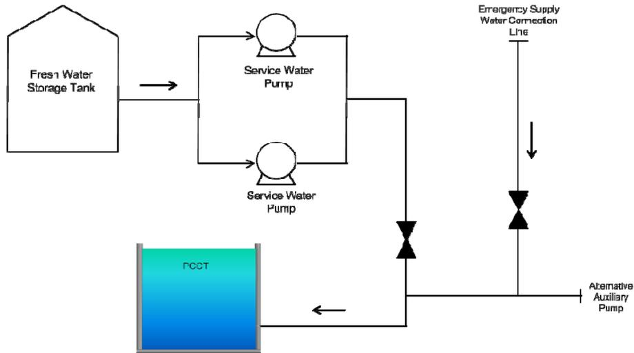
Fig. 2. Outline of Passive Condensate Cooling Tank Makeup Line
