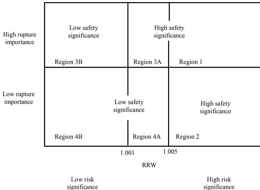
Fig. 1 Piping segment selection matrix in the modified WOG methodology
