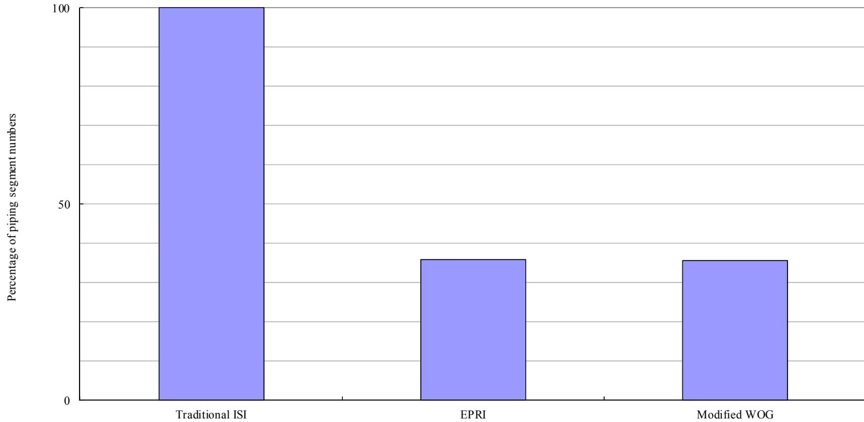
Fig. 2 Numbers of piping segments where surface or volumetric tests are required
