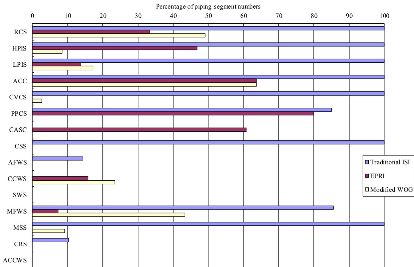
Fig. 3 Numbers of piping segments where surface or volumetric tests are required in each system
