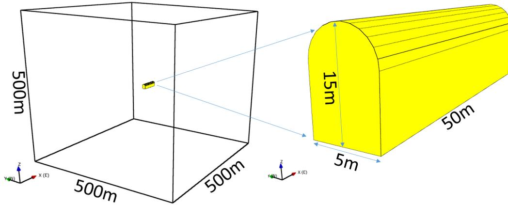
Fig. 1. Modeling area with a disposition tunnel for a hypothetical deep geologic HLW repository
