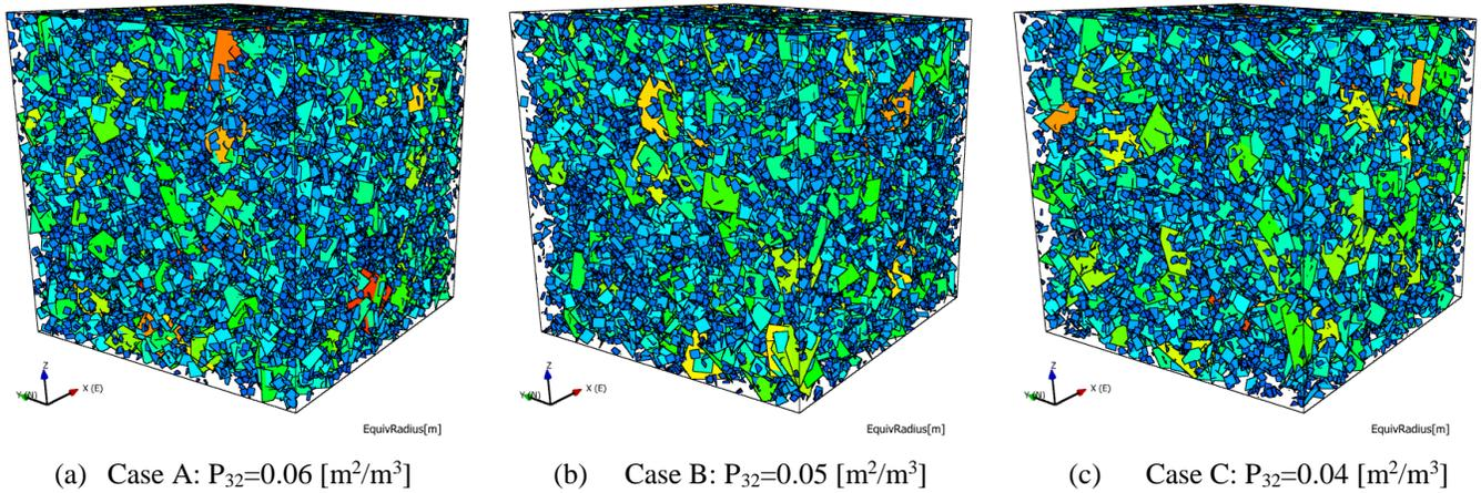
Fig. 2. A Particular Realization of Discrete Fracture Network for Three Fracture Systems
