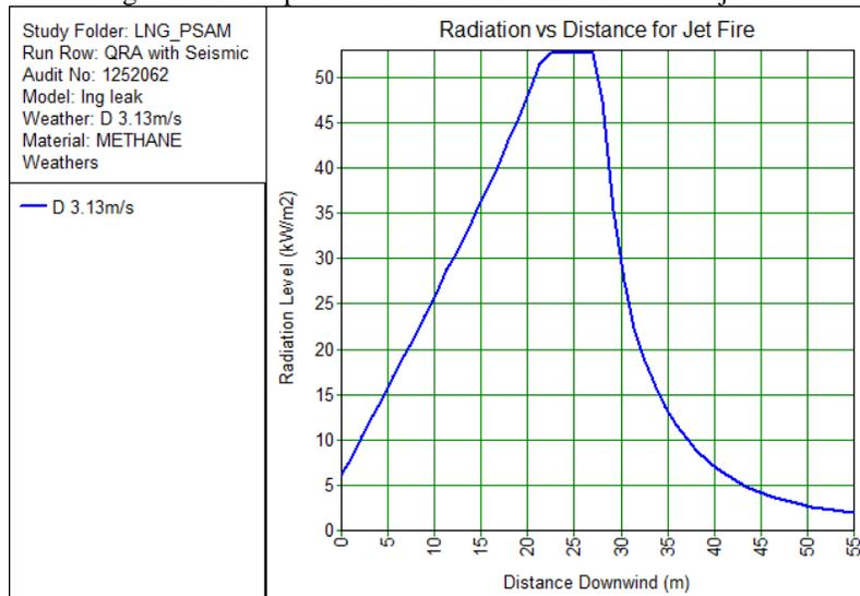
The adjacent tank distances of tank #1~8 are all about 30 m as in Figure XII. Therefore heat radiation level is approximately 30 kW/m<sup>2</sup> from Figure X.
