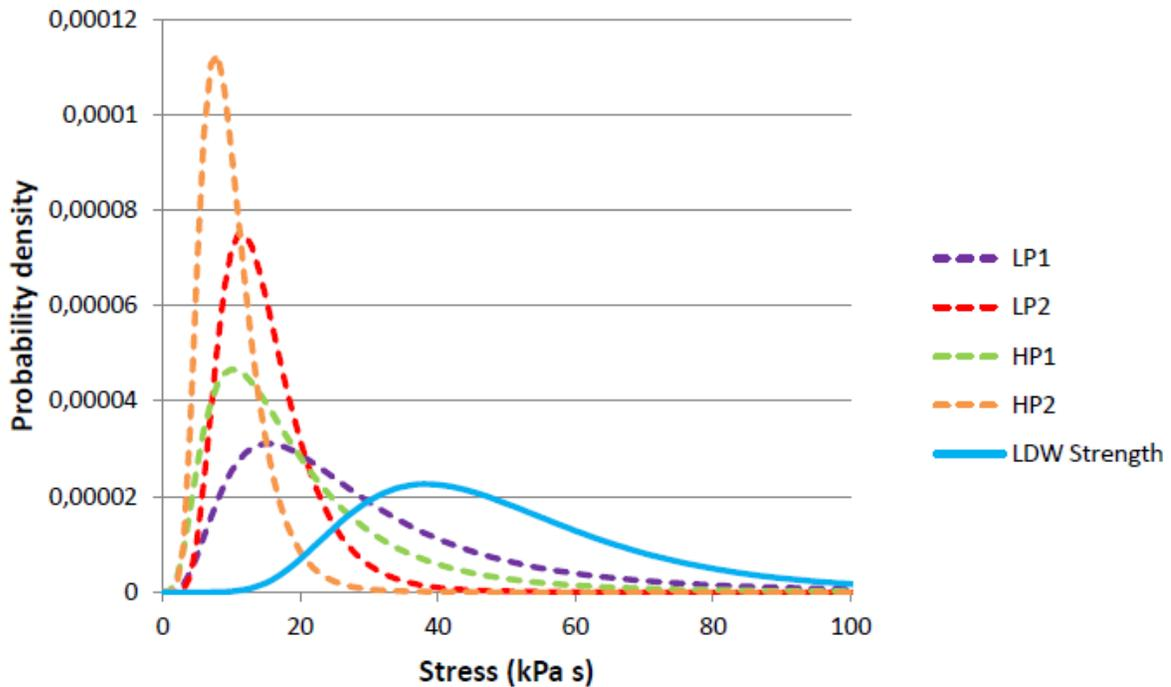
Fig. 1. Distributions used to determine whether LDW fails due to pressure impulse caused by ex-vessel steam explosion.
