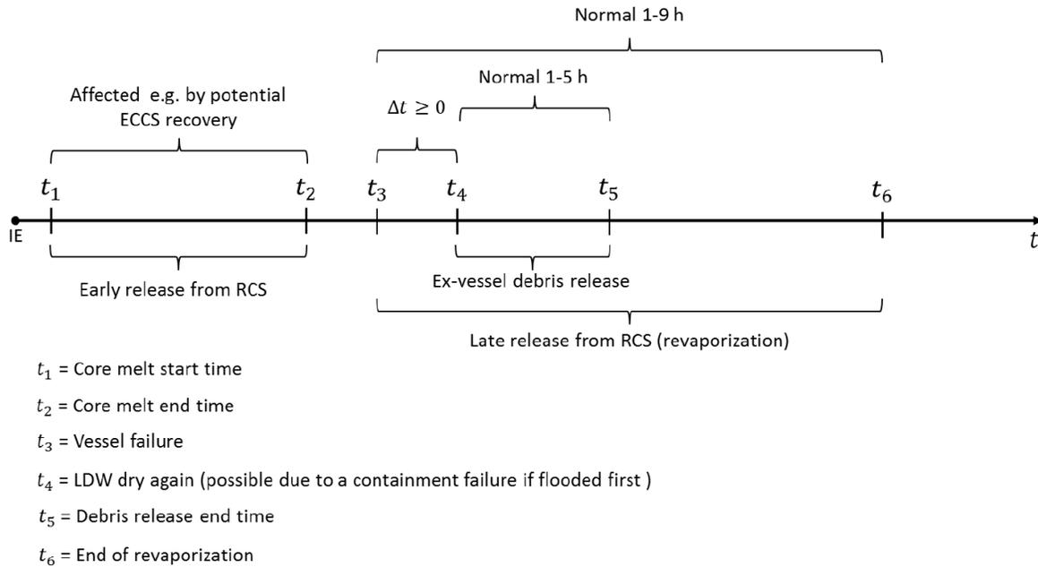
Fig. 4. The timings of the different release mechanisms.
