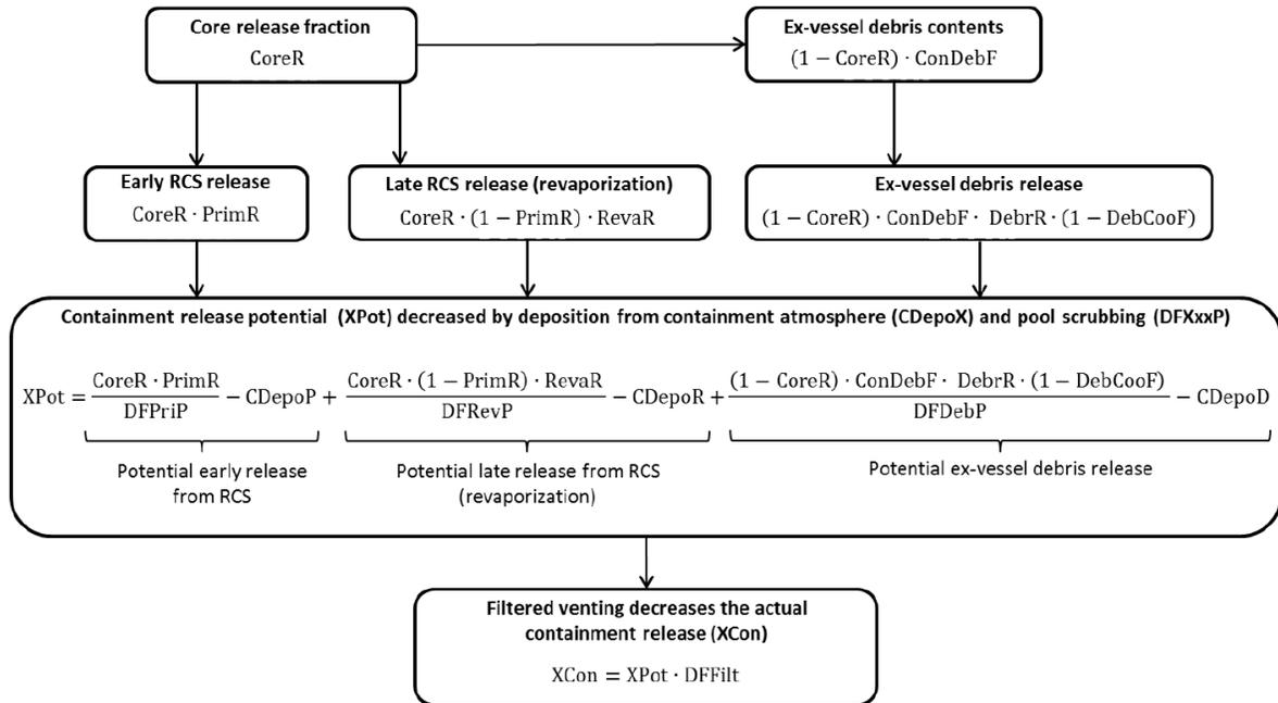
Fig. 3. Source term model that calculates releases out of the containment.
