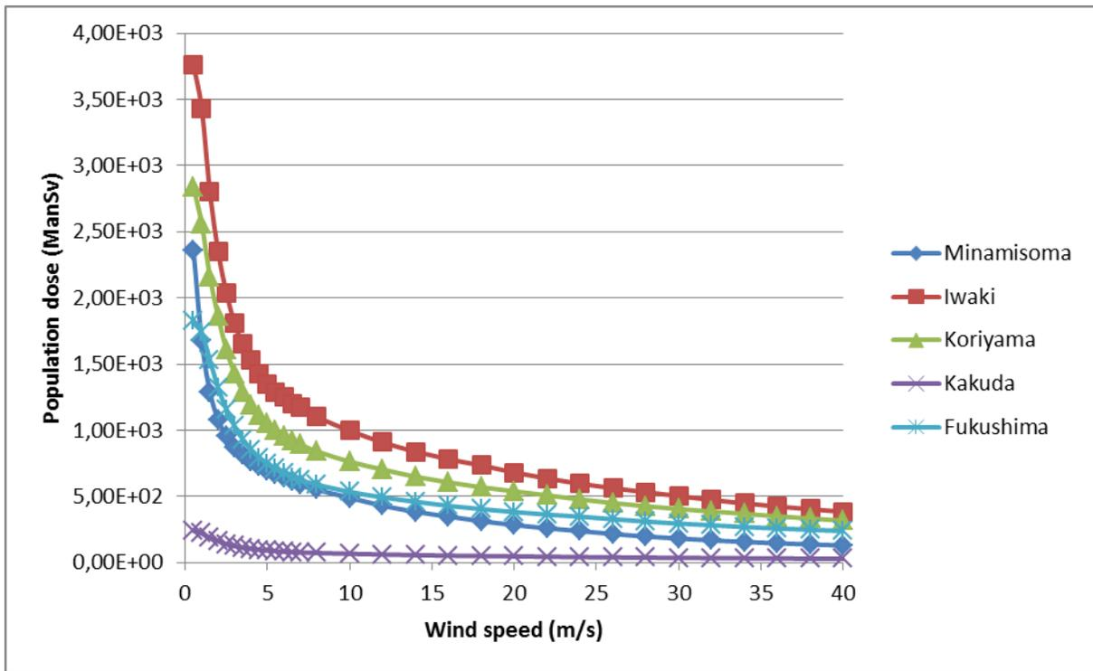
Fig. 2. The population doses calculated in ARANO as functions of wind speed in the case of no rain.
