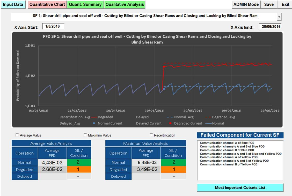
Figure 3 - Example illustrating the effect of the failure of both communication channels on Safety Function 1
