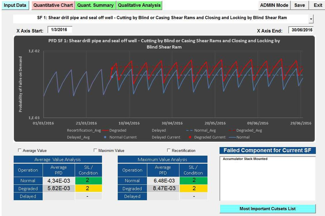
Figure 2 - Example illustrating the effect of the failure of the stack mounted accumulator on Safety Function 1
