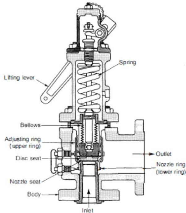
Fig. 2. Typical Crosby pressurizer safety vent valve model HB-BP-86<sup>18</sup>.
