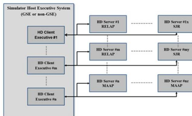
Fig. 3. Multiple client-server architecture<sup>23</sup>.
