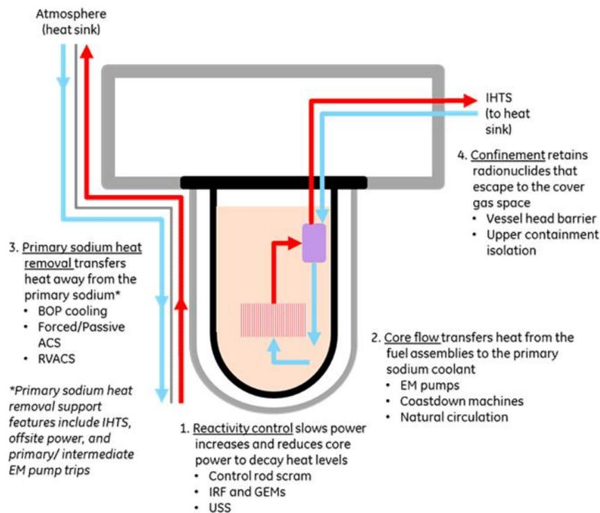
Fig. 5. PRISM PRA Safety Functions<sup>2</sup>
