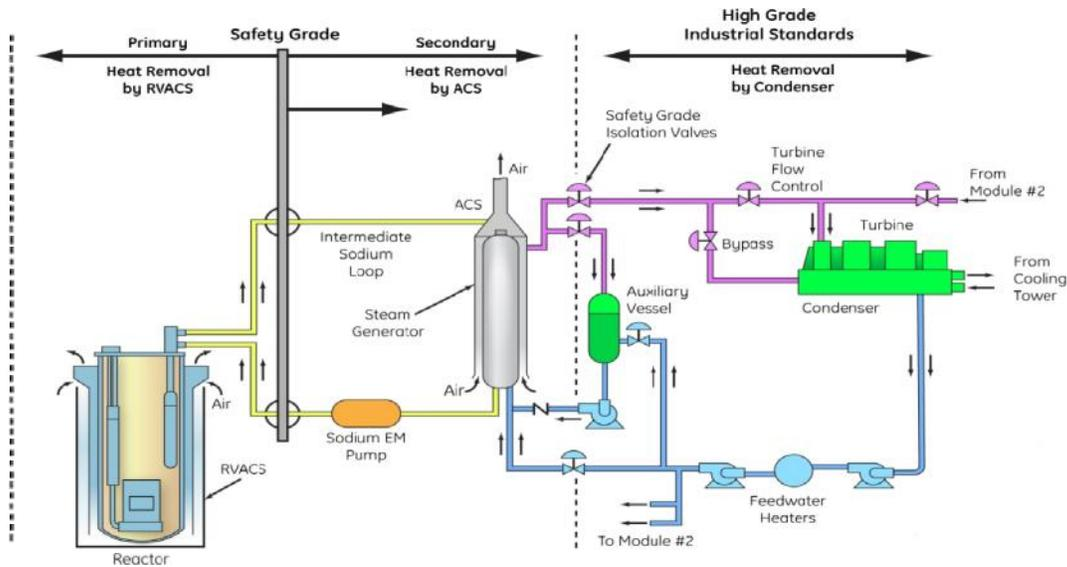
Fig. 2. PRISM nuclear steam supply system
