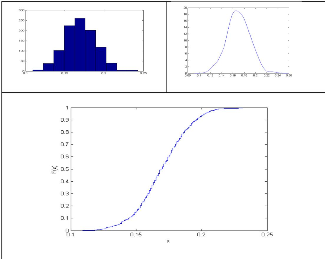
Figure 8: Monte Carlo generated uncertainty distribution for steam generator tube failure
