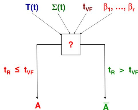
Figure 7: RCS component creep rupture parameters and criterion [3]
