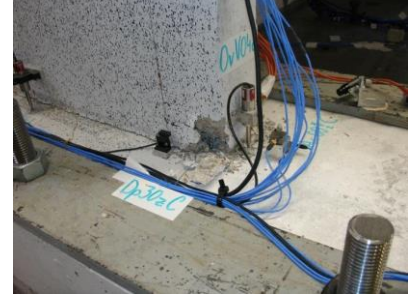
(c) Damage in the concrete wall
