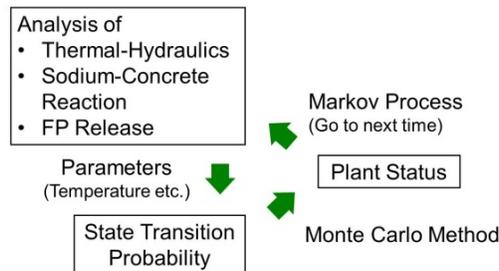
Fig.1 Concept of the CMMC coupling method
