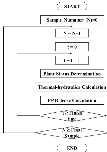
Fig. 3 Fission Product Transport Analysis Model Algorithm
