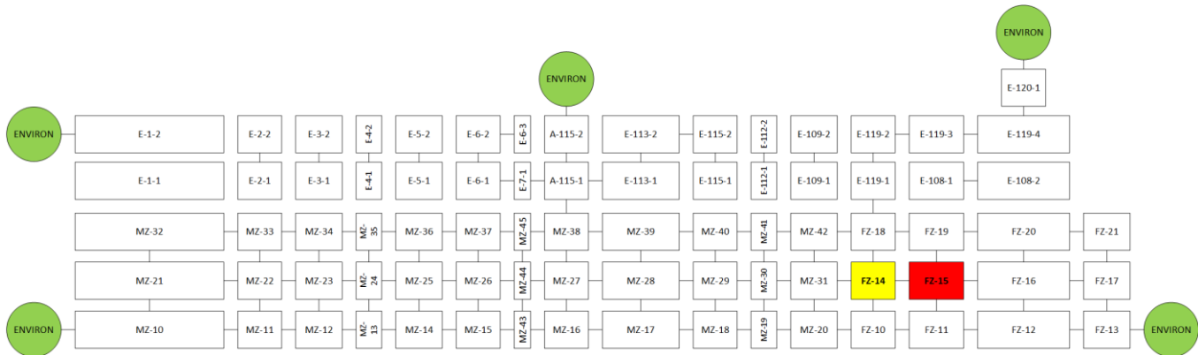
Fig. 7. COCOSYS computational model of the turbine hall and adjacent compartments
