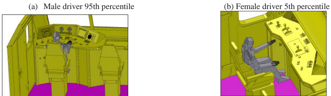
Fig. 5. Virtual scene of potential male driver 95th percentile (8200-class locomotive)
