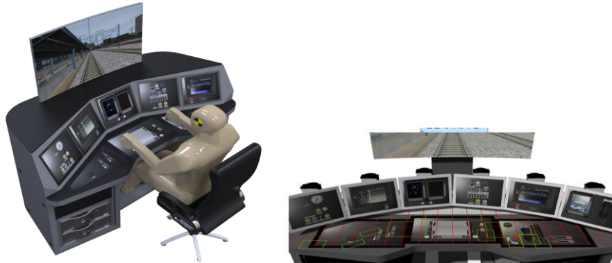
Fig. 9. Virtual engineering simulator for the driver-machine interface
