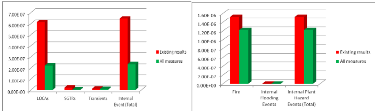
Fig. 5. Impact of plant modifications on CDF for internal events (left) and for internal plant hazard events (right).
