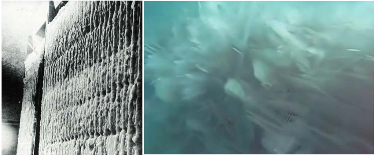
Fig. 2 and 3. Frazil ice in an experimental test rig (left) and frazil ice in seawater intake mesh grid (Ref 1.)
